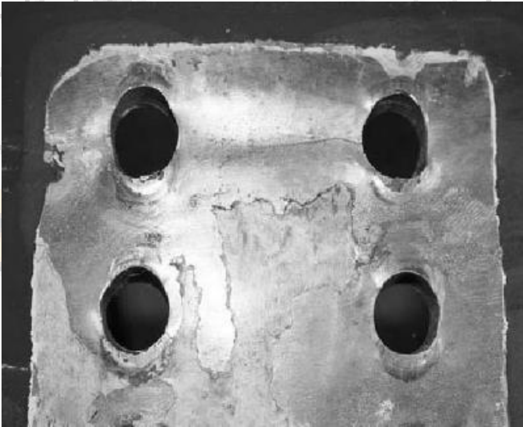
Figure 10.16 Bearing failure of plates
