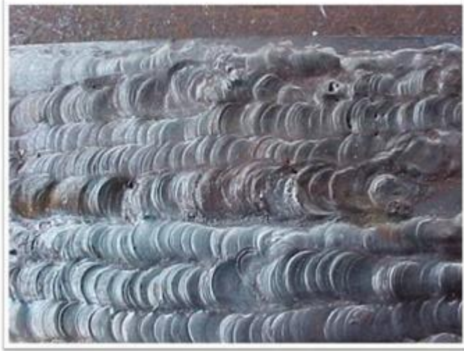
Figure 7.23 unacceptable weld profiles
