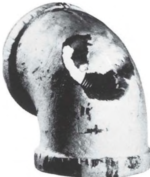
Fig. 5.12: Impingement failure of an elbow that was part of a steam condensate line.
