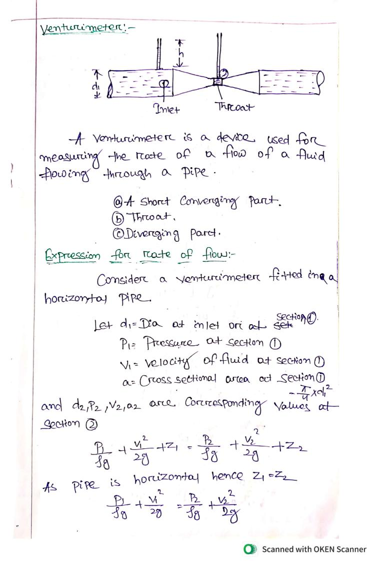
$$\frac{1}{3} \frac{P_{1} - P_{2}}{3} = \frac{V_{2}^{2}}{2g} - \frac{V_{2}^{2}}{2g}$$
