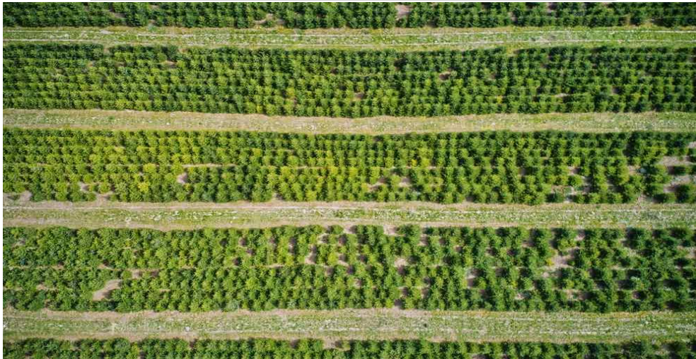
Vertical aerial photographs have no tilt in the camera axis.
